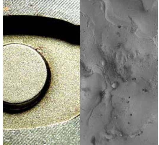
Figure 3 - Cavity EDMed with an electrode exhibiting consistent microstructure.
